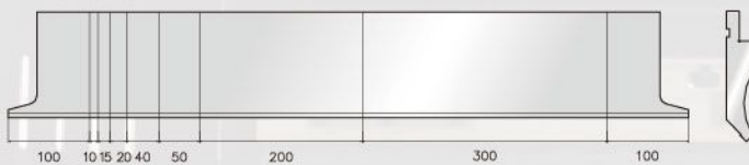
Segment diagram for upper mold
